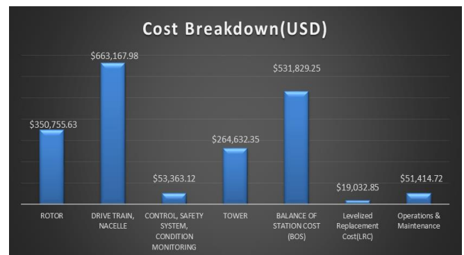
Fig.3. first test example cost break down
